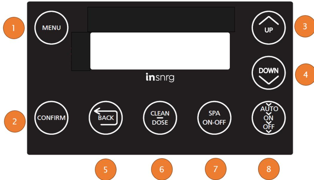
1. Go to INSTALLATION MENU (5) and turn INSNRG CHLORINATOR OFF>press CONFIRM.
