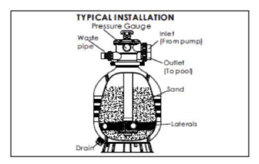
17) To prevent water leakage, be sure all pipe connections are tight 18) Prior to starting the filtration process by turning on the pump, we highly recommend that you read through the pump instruction manual to ensure proper installation and to avoid the risk of electric shock.
